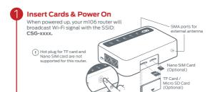
After Inserting cards, turn on the router by pressing the power button
